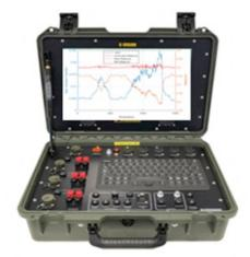
COR<sub>x</sub><sup>™</sup> Gas Void Fraction Monitoring Systems provide a practical means to accurately monitor gas void fraction levels in liquid outlets of separators over extended periods of time over which process and or production conditions can vary.
